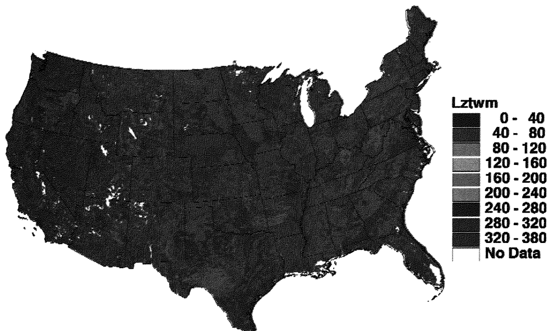
Figure 2. The lower layer tension water capacity derived from soil data for the conterminous US.
